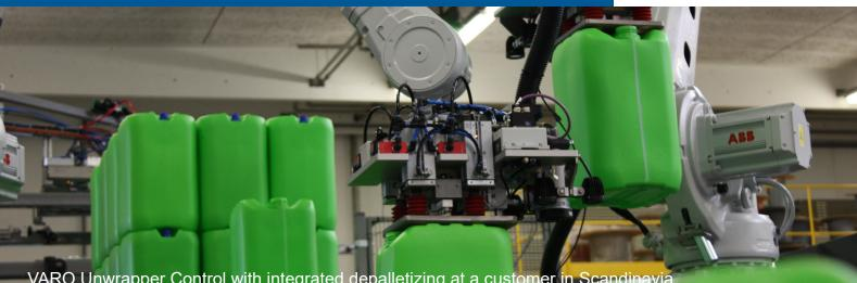
VARO Unwrapper Control with integrated depalletizing at a customer in Scandinavia
